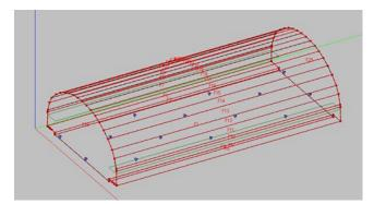
Figure 2 – Ease model of a section of the tunnel, showing the position of the sources.
