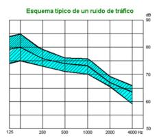
Figure 3 - Typical frequency spectrum of road traffic (SPL).
