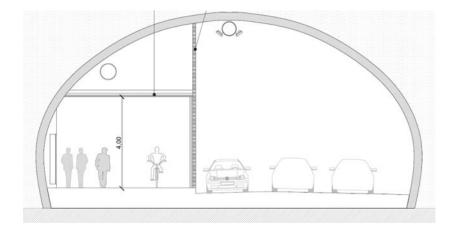
Figure 11 - Section of the proposed gallery with a suppressed lane
