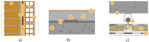
Figure 10 - Acoustic insulation a) Designed wall section b) Designed floating floor section c) Designed suspended ceiling section. Source: http://www.danosa.com/.
