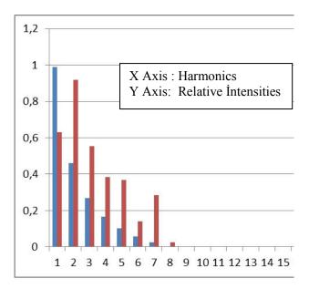
Figure 4. Red spectrum represents Electric Guitar. Blue spectrum represents Monocord's theoritical results
