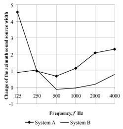
Figure 6 - Change of the azimuth sound source width for System A and System B.
