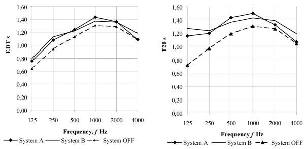
Figure 4 - Reverberation times EDT and T20 for two sound enhancement systems compared with the original value.
