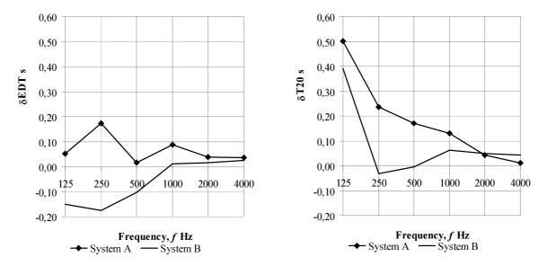
Figure 5 - Differences in EDT and T20 between ER and ALL operational mode for both systems.
