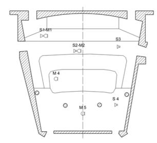
Figure 2 - Scheme of sound source and receivers locations in Rehearsal Room
