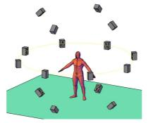
Figure 3 - Multichannel sound sources system in anechoic chamber
