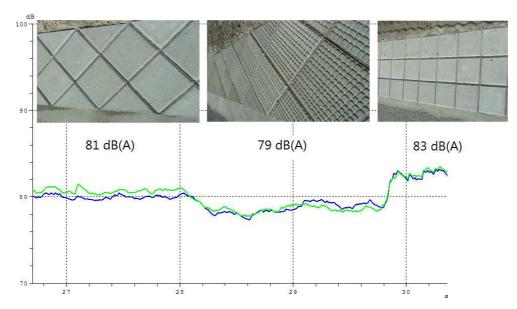
Figure 7 – Sound-pressure level of the tire/road-noise on different test tracks.
