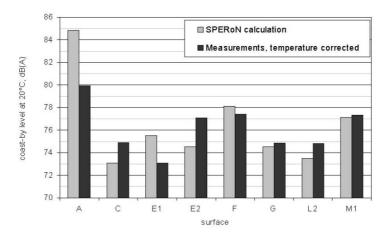
Figure 2 – Comparison of measurement and SPERoN calculation results depending on the surface for a velocity of 90 km/h.
