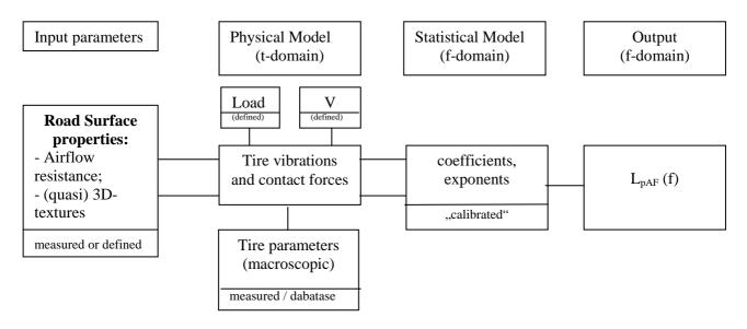
Figure 1 – SPERoN<sup>®</sup> structure (adapted from [6])
