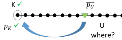
Figure 2 – One-dimensional acoustic domain, discretized in 15 coordinates, indicating the set U having one source pressure p_U (green triangle) and the set K having a measured pressure p_K (circle).
