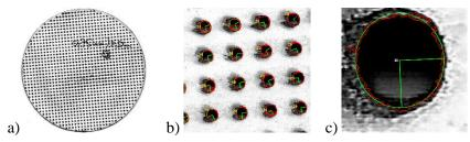
Figure 2 – Exemplification of image processing process: (a) original RGB image; (b) detected holes plotted in an extract of the original image; (c) zoom in of a detected hole (boundary of a hole represented in red and the approximated ellipse and their axis in green).
