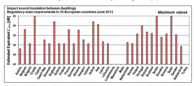
Figure 4 – Overview of impact sound insulation requirements between dwellings. Status 2013. Graphical presentation of estimated equivalent values of L'<sub>nT,w</sub>. Note: The equivalent values are estimates only, as exact conversion is not possible. Figure from [10].
