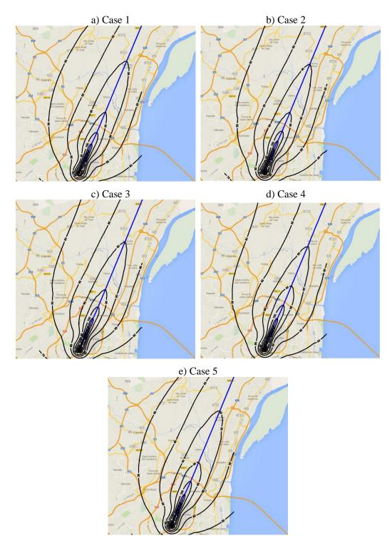
Figure 3 – Noise maps for the departure test cases, representing the aircraft's trajectory (blue line) and the SEL (in dB) contours (black lines).
