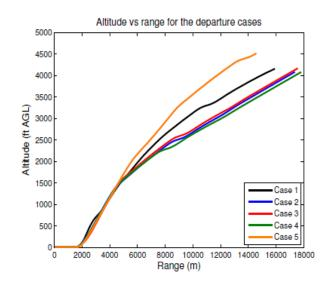
Figure 2 – Altitude as a function of distance to the start of take-off roll.
