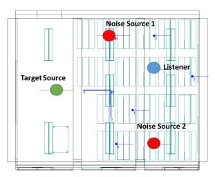
Figure 4 – The location of the target source, the two noise sources and the listener location in the classroom.
