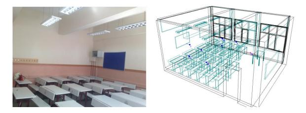
Figure 2 – The photo of the classroom showing the interior materials and the furniture. (Left figure). The ODEON wireframe model of the classroom. (Right figure)
