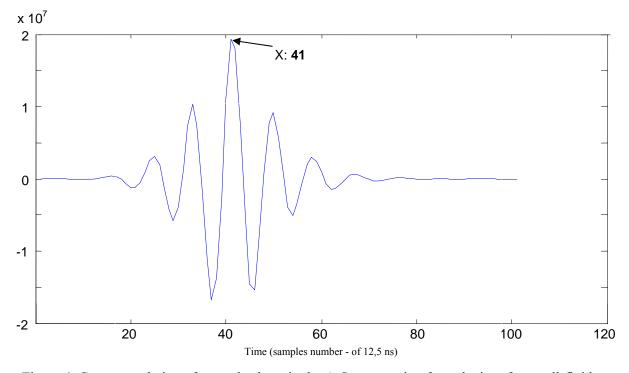
Figure 4. Cross-correlation of second echoes in the A-Scans coming from the interface wall-fluid.
