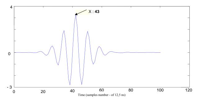
Figure 3. Cross-correlation of first echoes in the two A-Scans (coming from the interface fluid-wall)
