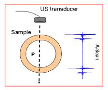
Figure 1. Scheme of the walls displacements measurement in a cylindrical tube. Each A-Scan contains 4 echoes, from the four sample-fluid interfaces.
