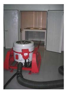
Figure 1 – Facility used during the test: An electrodynamic shaker was used for the vibration excitation. This was installed inside an acoustic enclosure to reduce the noise from the shaker inside the chamber. The measurements were carried out inside the CTAG anechoic chamber.
