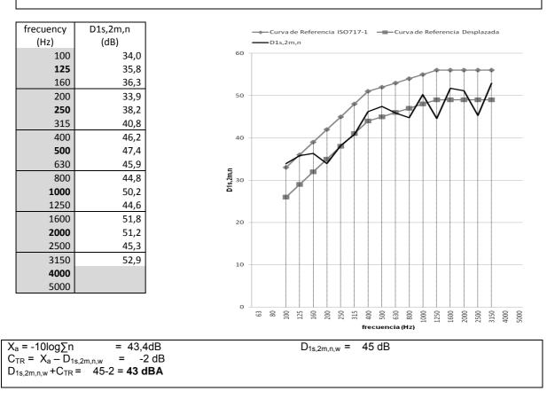
Using the same method, another measurement is done in a classroom. This façade is composed by 10 m2 of opaque multilayer wall with and 15 m2 of window. The sound level meter was always positioned at least 0.5m away from any room boundary or diffuser and at least 1m from the source. Each measurement position was at least 0.7m away from other positions where practicable and on a different axis.
