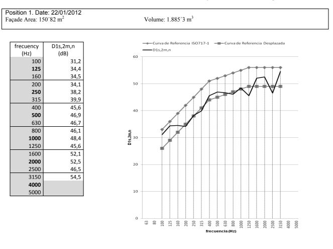
Table 2 results of Airborne Sound Insulation for active glass curtain wall in 3 positions.
