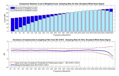
Figure 4.1: Comparison between measured Z and A-weighted levels for broadband white noise input signal.
