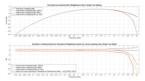
Figure 3.1: Theoretical and implemented A-Weighting filters for sampling frequencies at 44.1 kHz, 48 kHz and 192 kHz.
