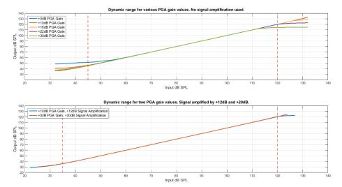
Figure 5.1: Linearity and dynamic range measurements for 0 dB, +10 dB, +16 dB, +22 dB and +30 dB PGA gain levels.
