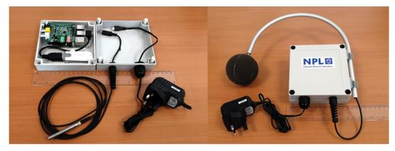
Figure 1: NPL's Raspberry Pi based wireless sensor network's measurement station.
