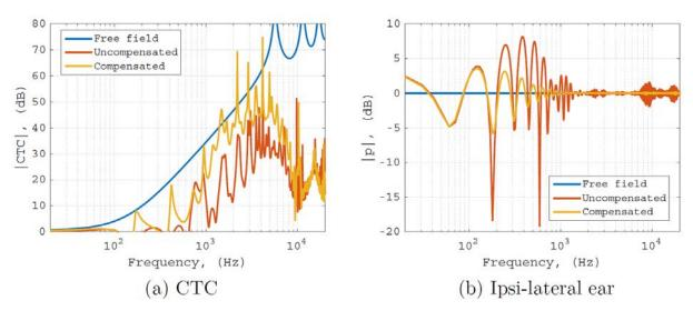
Figure 3: Cross talk cancellation and frequency responses under the effect of lateral reflections ("Uncompensated") and when these are compensated ("Compensated") compared with the free-field performance.
