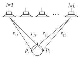
Figure 1: Geometry of the loudspeaker array used to control the acoustic pressure at the listener's ears.
