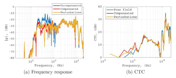
Figure 6: Measured frequency response and cross-talk cancellation performance in the setup of Fig. 5 for free-field filters (Uncompensated), compensation filters (Compensated) and compensated filters with modified wall distances to introduce errors (Perturbations).
