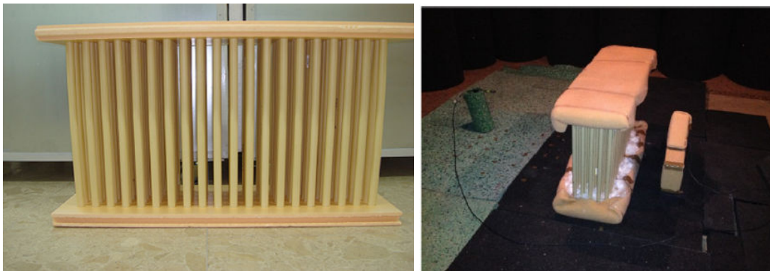
Figure 2 – a) Sample image of a 1:10 sonic-crystal prototype (from [14]); b) Image of the acoustic test.
