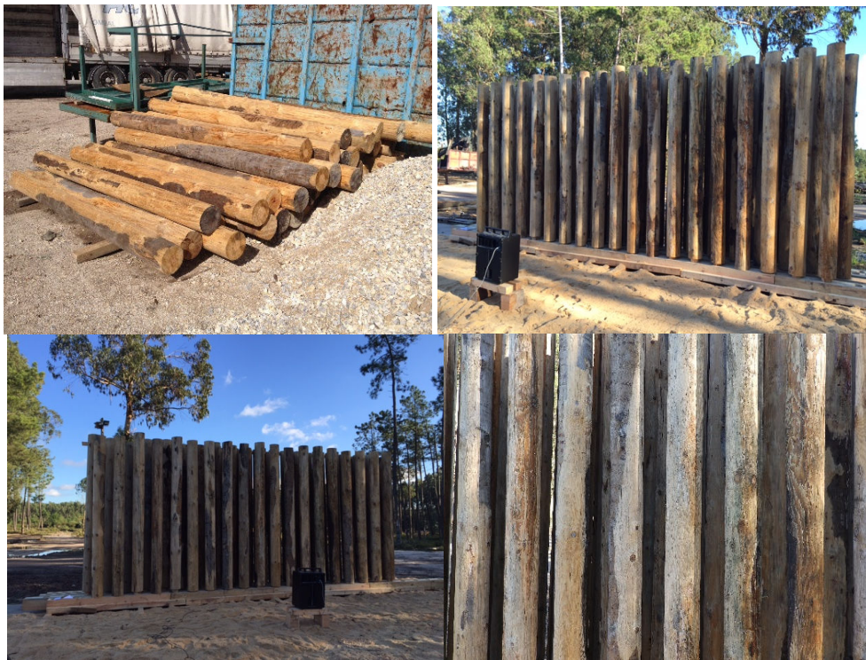
Figure 8 - Images of the timber logs and of the assembled prototype structure.
