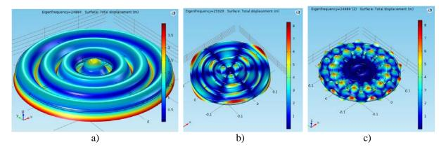
Figure 3 – Different vibration modes of the stepped circular plate. a) 7 nodal circles mode (24884 Hz).
