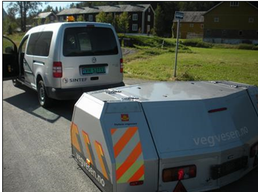
Figure 3 – CPX test trailer used by SINTEF.
