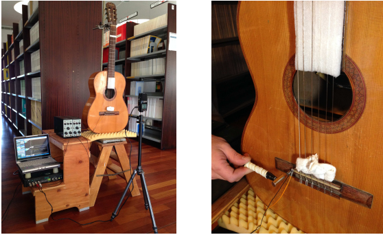
Figure 6: Measurement of the vibro-acoustic response of the tested guitar. Global view (left), impact testing measurement (right).
