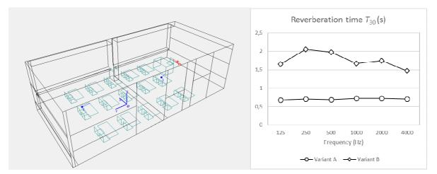
Figure 1 – Virtual model of classroom used for simulations. Two different reverberation time values  $T_{30}$  were used.
