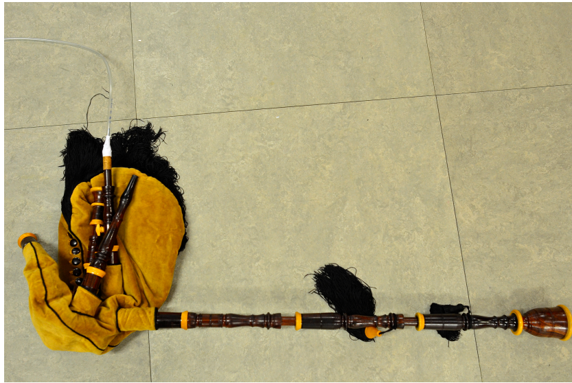
Figure 1 – Galician bagpipe without the melodic pipe, fitted with a pressure transducer on one of the small drones. The large drone (C3) was either opened or closed depending on the extract played.
