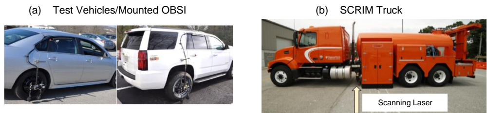
Figure 2 – (a) Test Vehicles, (b) SCRIM Truck.
