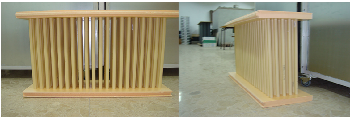
Figure 2 - Example of a tested noise barrier (1:10 scale model).
