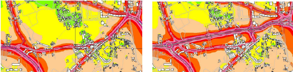
Figure 5. Comparison of noise maps for scenarios regarding road traffic changes; previous (left); future with new traffic diversion (right).
