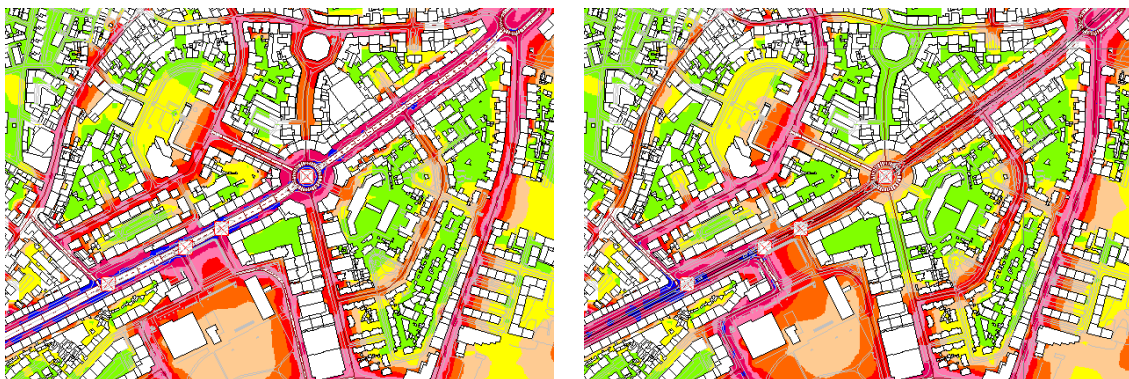
Figure 4. Samples of noise maps of an urban area, before (left) and after (right) implementation of noise mitigation measures
