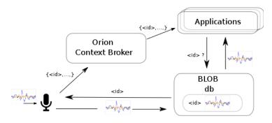
Figure 6: Processing events and saving sound bites to a binary large object (BLOB) storage database.
