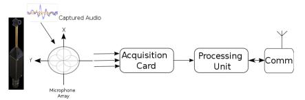
Figure3: FI-Sonic Sound Acquisition Module (Architecture).
