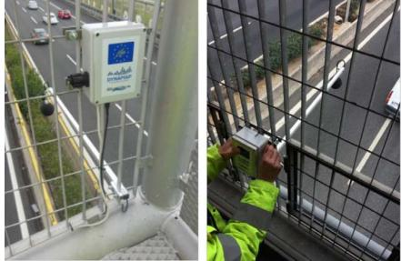
Figure 3: View of the Hi-Cap sensor installed in a portal of the A90 motorway in Rome
