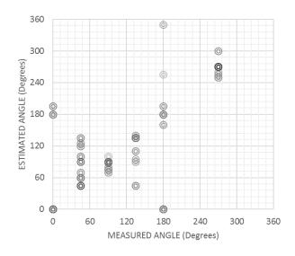
Figure 6. Azimuth answers for the voice synthesised with the HRIR of the microphones.
