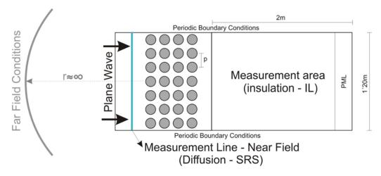
Figure 1: Numerical domain used for SCASAD simulations
