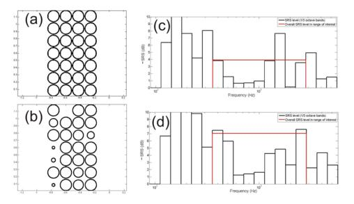
Figure 4: Scheme of the design of both (a) Reference Sonic Crystal and (b) Selected SCASAD (blue and green points in Figure 2, respectively); (c) and (d) Diffusion properties of both individuals respectively
