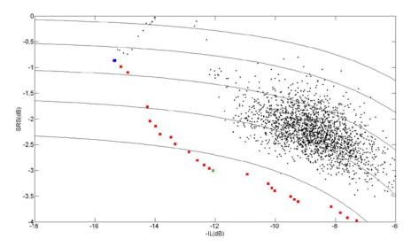
Figure 2: Objectives Space of the optimization done. The initial population (black dots), the Pareto Front (red dots), the most balanced individual selected (green point) and the reference individual (blue dot) are represented according their values of IL and SRS indexes.
