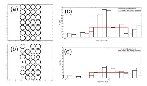
Figure 3: Scheme of the design of both (a) Reference Sonic Crystal and (b) Selected SCASAD (blue and green points in Figure 2, respectively); (c) and (d) Insulation properties of both individuals respectively
