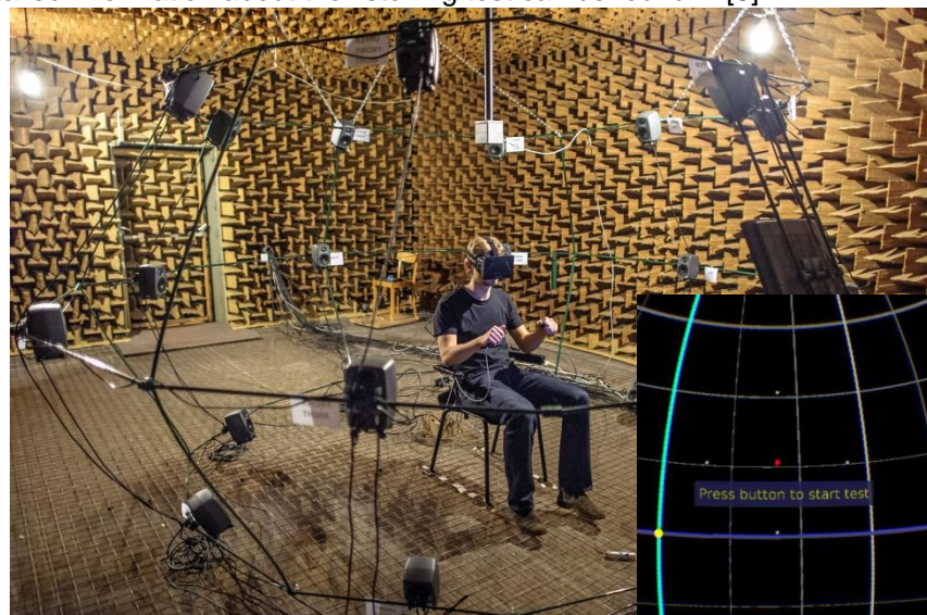
Figure 6: Listening test set-up and view in the HMD
