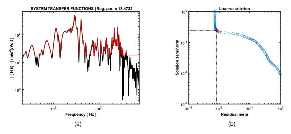
Figure 8: (a) comparison of the original (black) and regularized (red) electromechanical transfer functions. (b) corresponding L-curve for a logarithmically distributed range of regularization parameter.
