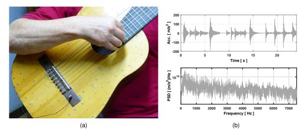
Figure 4: Live playing recording (a) and representative acceleration signal measured at the bridge (b).
