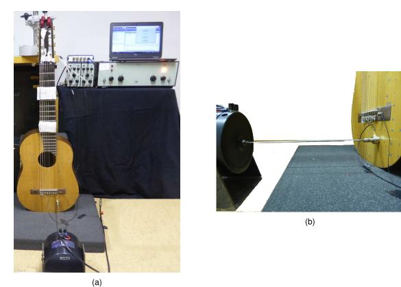
Figure 5: Experimental set-up for vibrating the guitar. (a) Global view with the PC controler, the acquisision module, the amplifier and the shaker; (b) detail of the shaker mounting with the force transducer and accelerometer.
