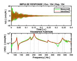
Figure 2: Measured (green) and reconstructed (red) impulse responses and transfer functions at the bridge. Dotted lines stands for the identified modes.
