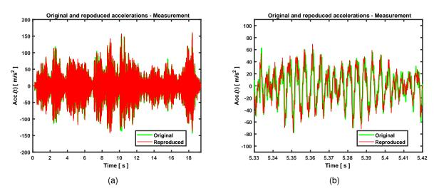
Figure 9: Experimental results. Comparison of the target and measured acceleration. Global time history (a) and temporal zoom (b).
