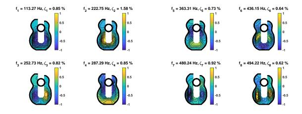
Figure 3: Modal frequencies, modal damping value and mode shape for the principal lower-order modes.
