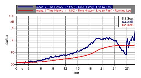
Figure 2: Sound pressure level and equivalent continuous level
