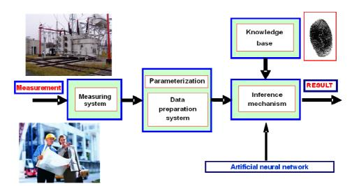
Fig. 2 Block diagram of the ES based on the AE method making it possible to assess the aging degree of the power transformer insulation system
