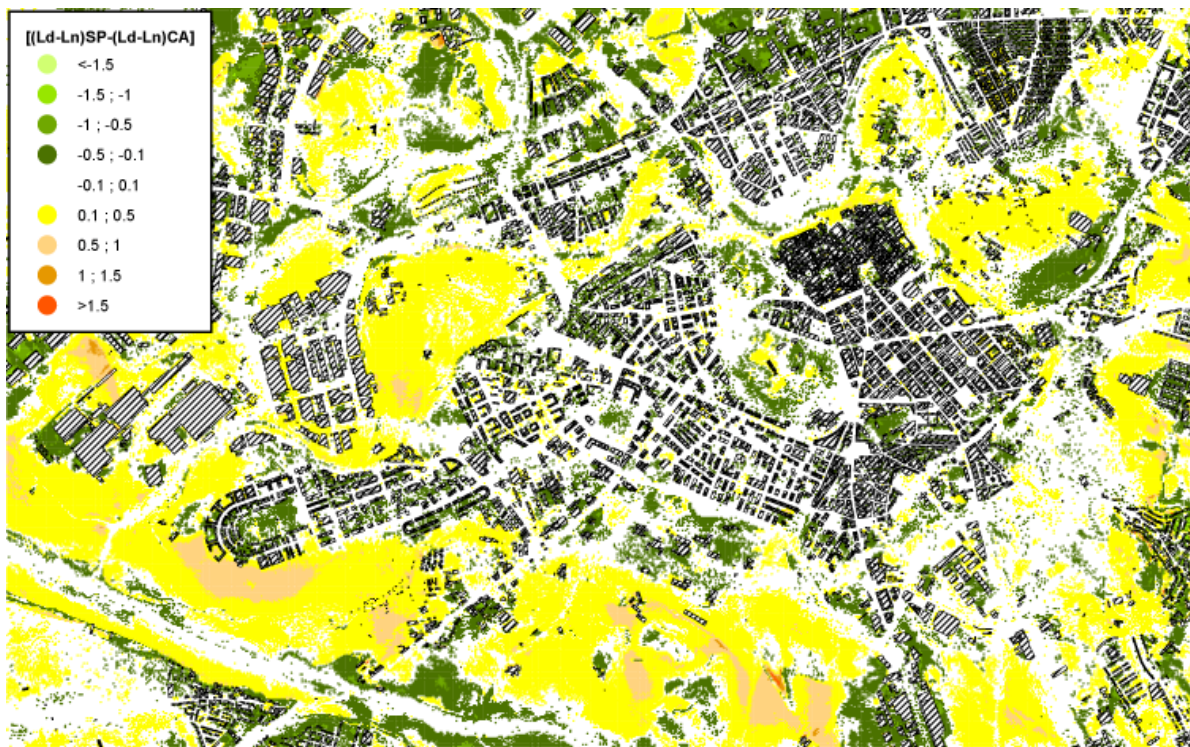
Fig. 5 – Differences between favorable and homogeneous atmospheric conditions from both programs, [(Ld-Ln)_{SP}-(Ld-Ln)_{CA}] , in dB.
