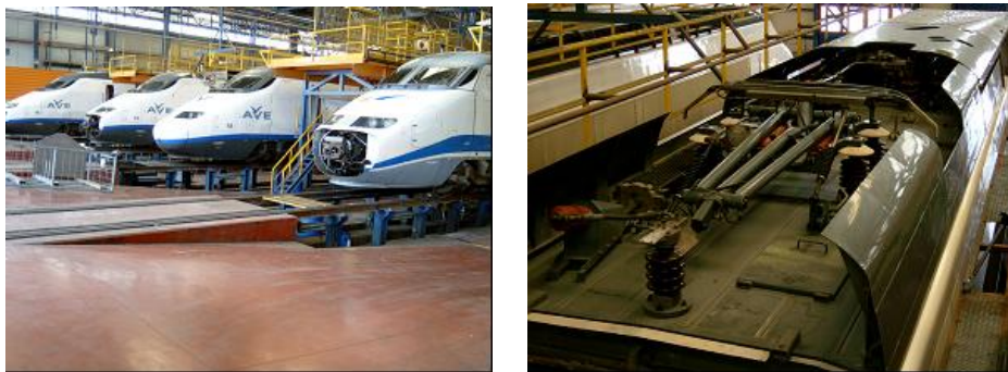
Figure1 (a): Measured AVE units. (b) Detailed view of the pantograph
