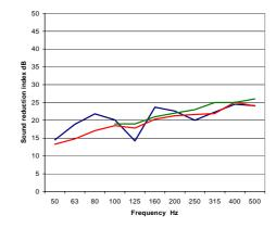
Figure 10 - Sound reduction index of a 12-mm fibreboard \_\_\_\_\_polynomial calculation, \_\_\_\_\_sinusoidal calculation \_\_\_\_\_measurement
