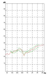
Figure 3 - Hollow brick wall modal theory, — measurements
