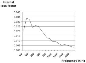
Figure 7 - Loss factor as a function of frequency
