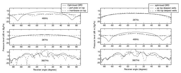
Figure 3 – Far-field polar responses of optimised QRDs with lower frequency response (a) all wells with added elements and (b) only deepest wells with elements.
