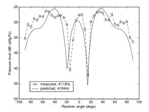
Figure 6 – Polar response of shallower diffuser with foil membrane.
