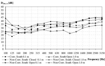
Figure 8 - Test cells' sound insulation – Case 3
