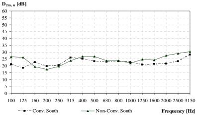
Figure 6 - Test cells' South walls sound insulation - Case 1
