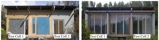
Figure 5 - View of the Test cells' without and with the glazed balcony
