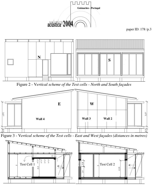
Figure 4 - Vertical sections of Test cells 1 and 2 (distances in metres)
