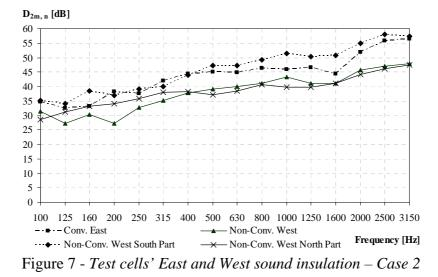
The non-conventional test cell South part of West wall and conventional test cell East wall, without windows and with the higher mass, are the walls that have the higher weighted normalized airborne sound insulation index, and a similar behaviour, as Figure 7 shows.
