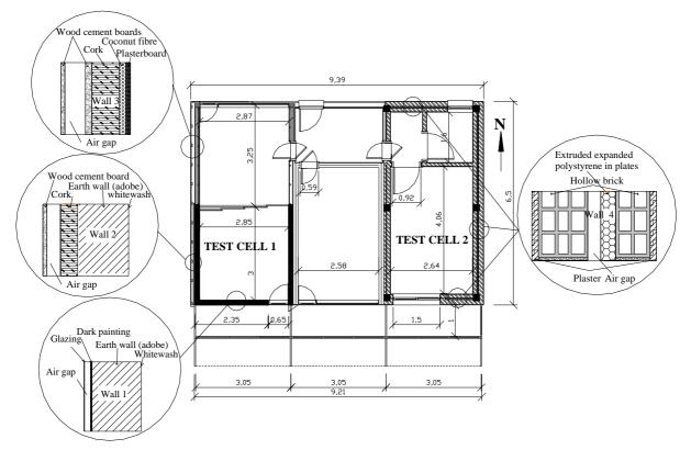
Figure 1 - Schematic plan of the Test cells and schematic section of some envelope components (distances in metres)
