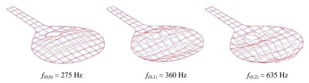
Figure 6 – Modeshapes of three resonances of the soundboard of guitar D.
