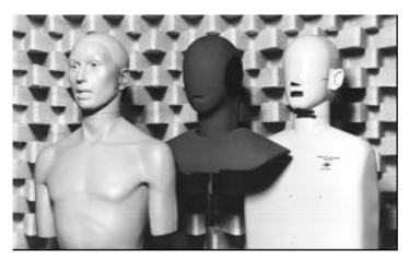
Figure 1 – Dummy heads (left to right): KEMAR, Head acoustics HMS II, B&K 4128
