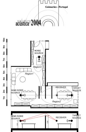
Figure 1 - Ground floor and section of the room (ceiling height is 2.7 m)
