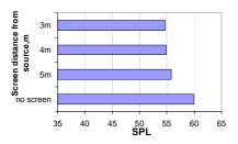
Figure 2 - Effect of position of screen (2x2 m screen)
