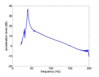
Figure 3 - Typical resonant curve with sine sweep excitation
