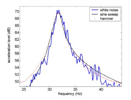
Figure 5 - Resonant curves with the three different excitation methods
