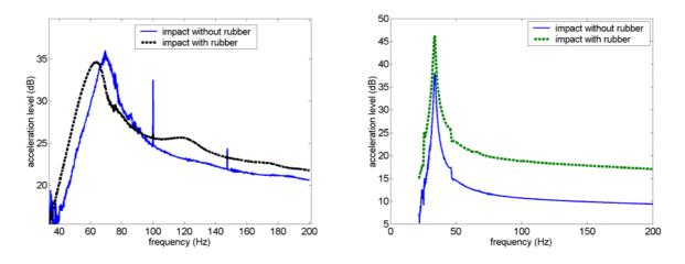
(a) Treated Rubber (6.3 mm thickness)
