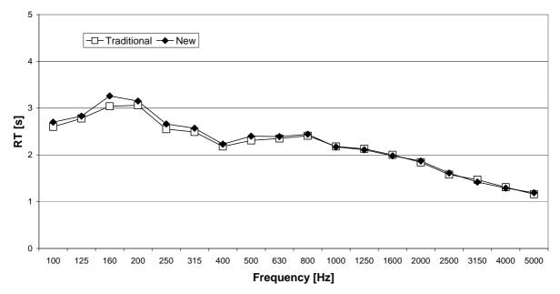
Figure 3 - Reverberation Time. Comparison between New and Traditional techniques
