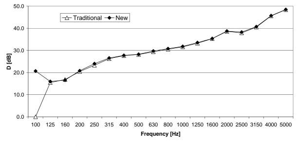
Figure 5 - Level difference. Comparison in high extraneous noise condition
