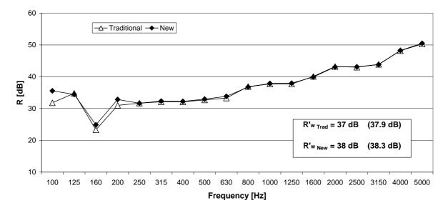
Figure 4 – Apparent Sound Reduction Index. Comparison between New and Traditional techniques
