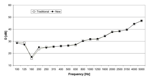
Figure 2 - Level difference. Comparison between New and Traditional techniques
