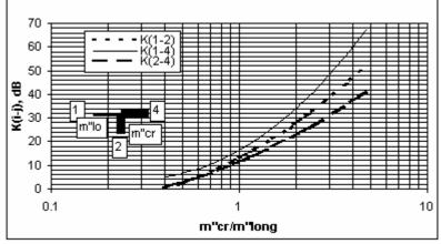
Fig 1. K<sub>ij</sub> of asymmetric T form junction
