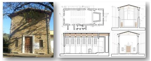
Figure 5: The church of Rispescia. facade, plan, elevations and sections.
