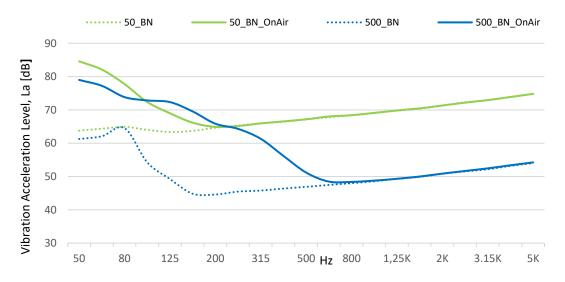
Figure 3. BN\_OnAir experiment  $L_a$  and BN\_OnRubber (50\_BN and 500\_BN) experiment  $L_a$  comparison, with 50mV/g and 500mV/g sensors.
