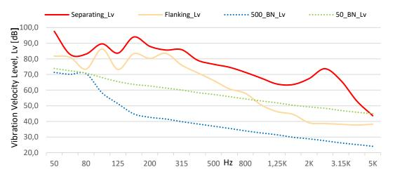
Figure 2. Separating element  $L_v$  and flanking element  $L_v$  comparison versus measurement system inherent noise  $L_v$  with 50mV/g and 500mV/g sensors performing BN\_OnRubber experiment.
