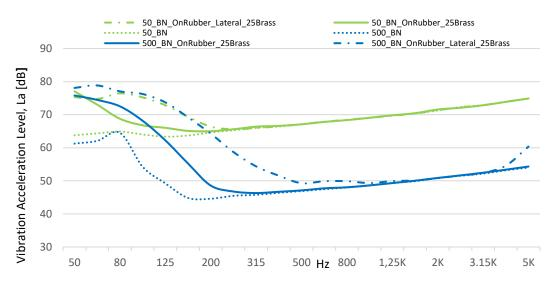
Figure 6. BN\_OnRubber\_25Brass La, BN\_OnRubber\_25Brass\_Lateral and BN\_OnRubber (50\_BN and 500\_BN) experiment La comparison with 50mV/g and 500mV/g sensors.
