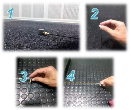
Figura 1. Example photographs on some postitions: 1) BN\_OnRubber, 2) BN\_OnAir, 3) BN\_OnRubber\_6.5Brass\_Lateral, 4) BN\_OnRubber\_255Brass\_Lateral
