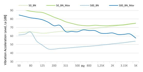
Figure 4. BN\_Mov experiment L<sub>a</sub> and BN\_OnRubber (50\_BN and 500\_BN) experiment L<sub>a</sub> comparison with 50mV/g and 500mV/g sensors.
