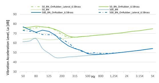
Figure 5. BN\_OnRubber\_6.5Brass L<sub>a</sub>, BN\_OnRubber\_6.5Brass\_Lateral and BN\_OnRubber (50\_BN and 500\_BN) experiment L<sub>a</sub> comparison with 50mV/g and 500mV/g sensors.
