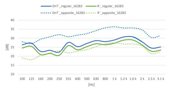
Figure 4. Airborne sound insulation ratings comparison, according to ISO 16283-1, both ways.
