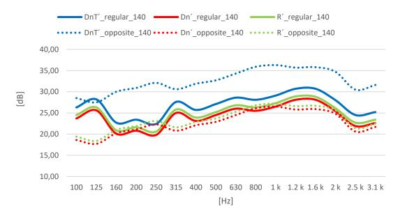
Figure 3. Airborne sound insulation ratings comparison, according to ISO 140-4, both ways.
