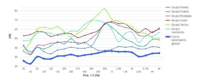
Figure 5. Walls sound transmission lost contribution comparison by Solidnoise® method, and its software Noiselab®, regular way.
