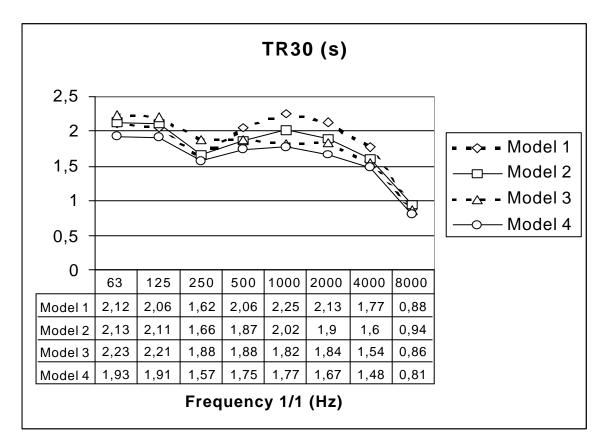
Fig. 4 Results obtained (TR30) from Odeon for different octave bands in the four simulations
