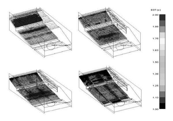
Fig. 5 Results for EDT at 500 Hz octave band from Raynoise in the four simulations
