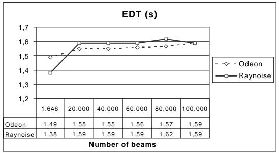
Fig.1 Values for Early Decay Time versus number of beams.
