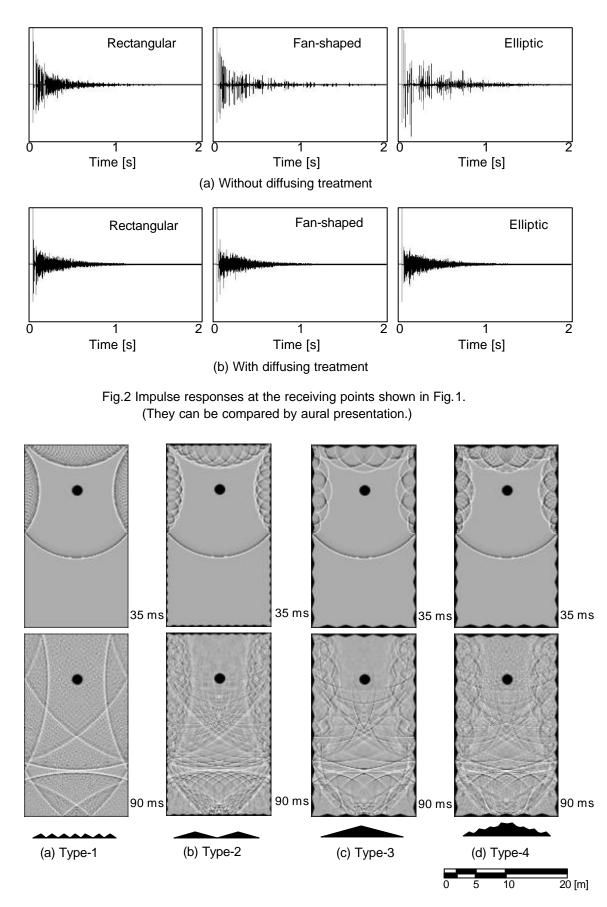
Fig.3 Comparison of sound propagation in the rectangular room with four types of diffusing treatments
