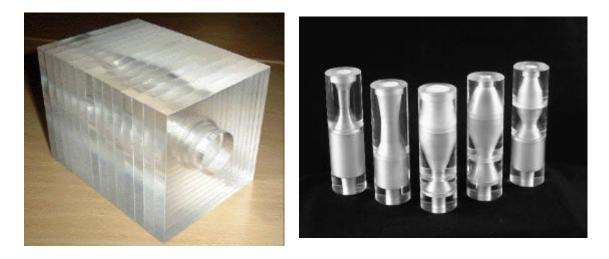
Fig. 3.- Two types of mechanical models of the human vocal-tract (from Arai, 2001 [10])
