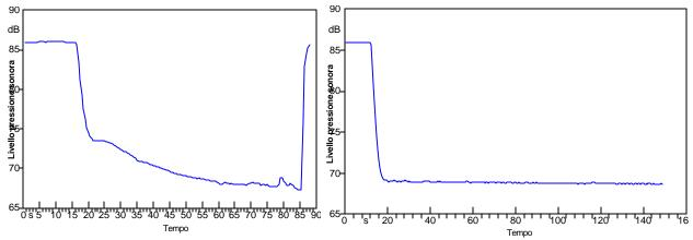
Fig. 3 – SPL reduction obtained with the active window (three loudspeakers and three microphones): left in laboratory; right in the experimental building.
