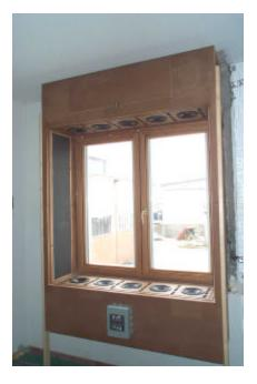
Fig. 2 – Active window: in laboratory (left) and in the experimental building (right).
