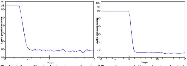
Fig. 6 – Active partition four-loudspeakers configuration; SPL waveform recorded by a microphone located in the receiving room. Left reverberation adjustment, right sound insulation.
