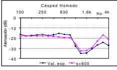
Fig.7.- Sound attenuation for wet grass. Theoretical (**s**=800 )and experimental.
